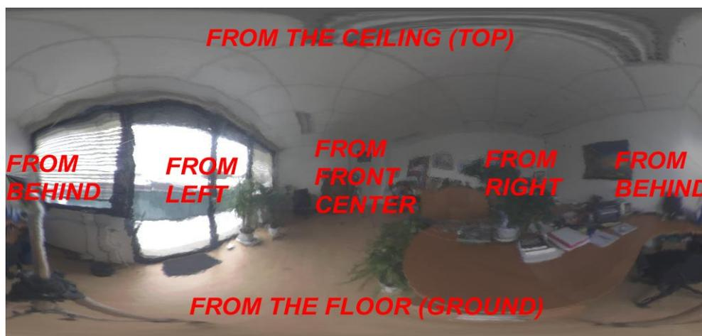
This image indicates which sections of the light probe will illuminate objects in the scene as seen from the point of view of the camera. Imagine this wrapped on a giant sphere around the scene.
